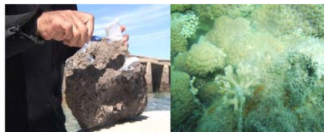
Figure 3 The slag shape before emerged (left) and after emerged in water illustrating the difficulty to distinguish between it and natural stone
