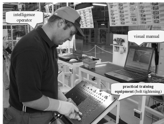
Fig. 7 Practical training scene using visual manual (bolt tightening)
