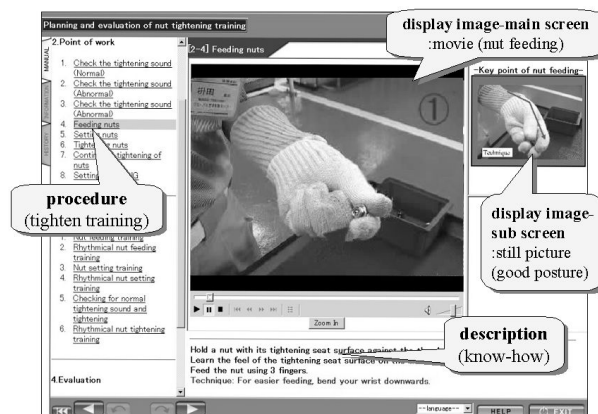
Fig. 6 Application example of V-MICS-VM-FSA (bolt tightening)
