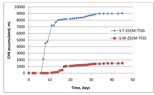
Figure 4  $CH_4$  accumulated for mesophilic (S-M-25CM-75SS) and thermophilic (S-T-25CM-75SS) tests
