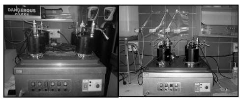
Figure 2 Experimental equipment used in the stirred biodegradability tests:mesophilic (left) and thermophilic (right)
