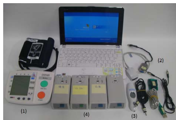
Fig. 1 Devices and sensors for measuring vital signs: (1) Sphygmomanometer, (2) Pulse oximeter, (3) Thermometer, (4) ZigBee-based devices
